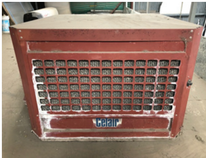
Calcium build up shows where water has been leaking from this cooler.
