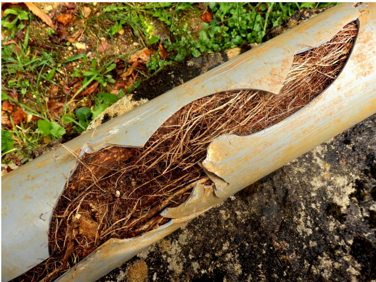
Tree root damaging stormwater drain
