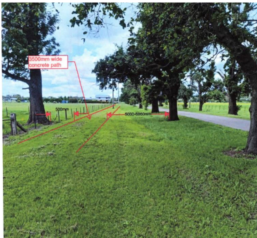
(Fig 7) Option 2 Adjacent to the fence line with the overhead power relocated: Option 2 would see the overhead power line relocated by either burial or moving the lines to the poles on the North- eastern side of the avenue, the path located 500mm offset the fence line, approximately 5m path edge to the centre of the tree line.
